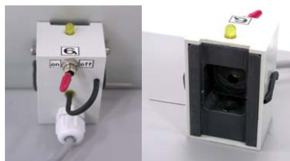
Module 6 – configured for tubing connection to the ultra-precise syringe-based liquid-dispenser
