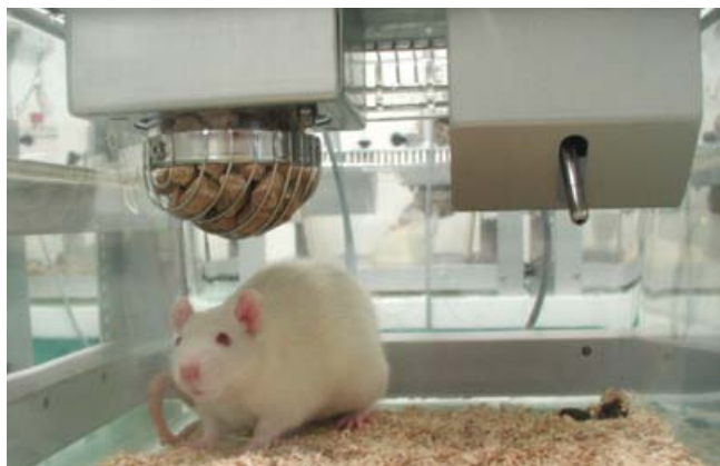
Rat in a home cage equipped with 1 Drinking & 1 Feeding sensor and placed into a MoTil frame
