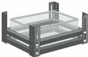
Home cage with infrared light-beam frame
