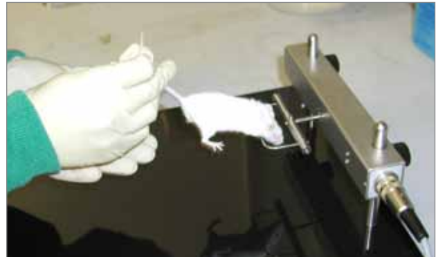
Sensor module shown with grasping grip for mice
