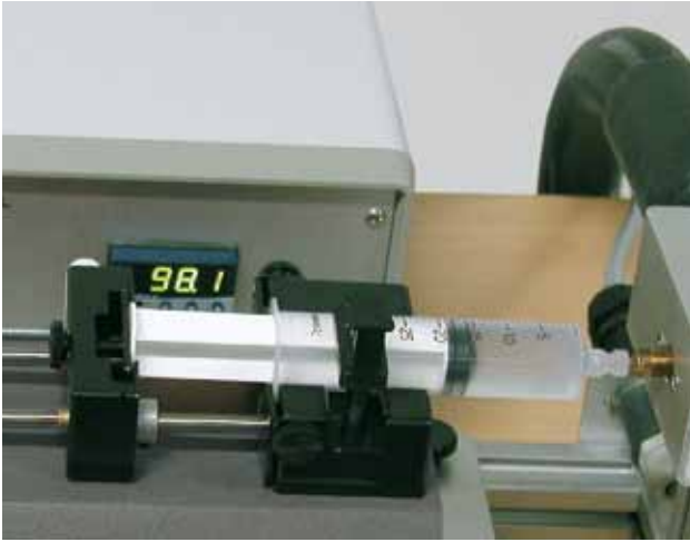
Vapor generator for volatile organic compounds (VOCs)
