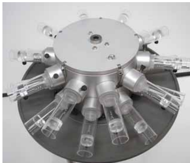
Head Nose Only Unit with one segment
