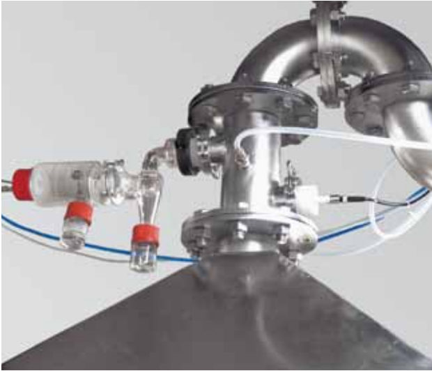
Aerosol conditioning line for Whole Body Unit
