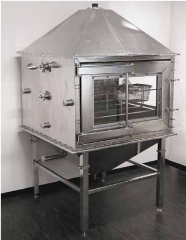
Whole Body Unit with a volume of approx. 0.95 m 3
