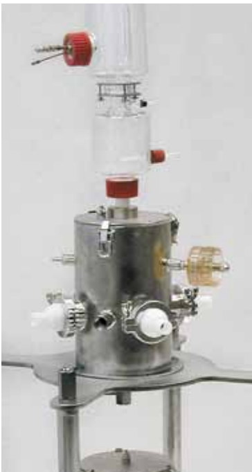
Upper unit with sample filter unit
