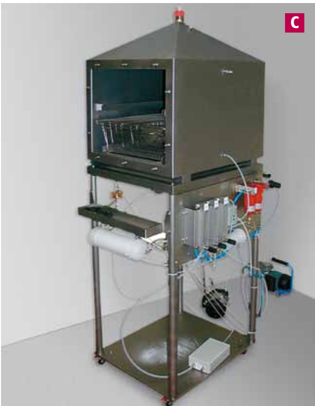
Whole Body Unit for one type 3 cage
