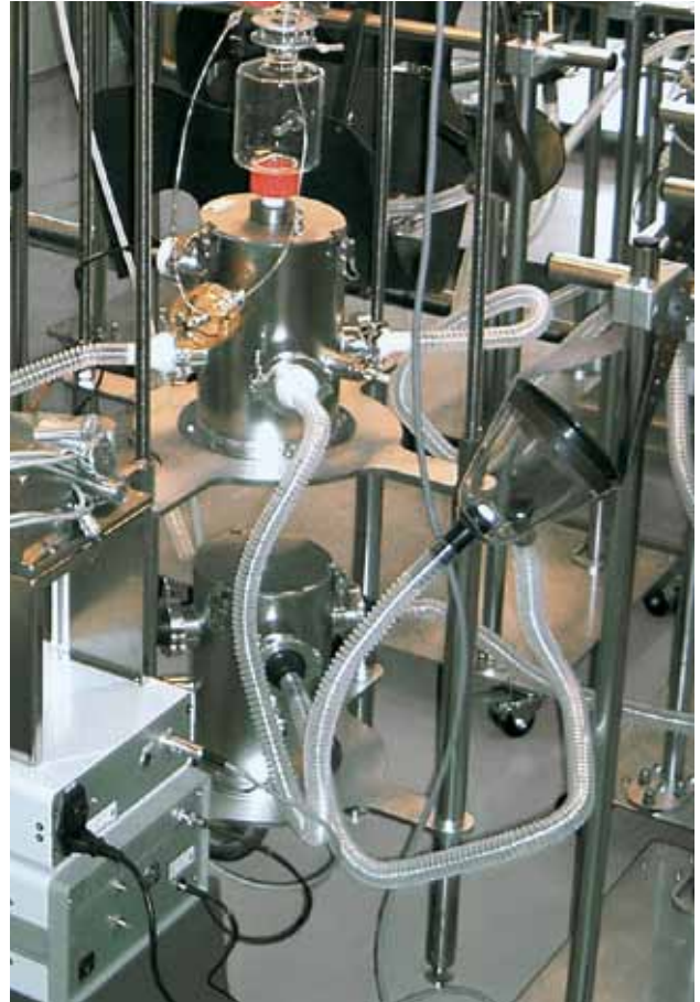
Dog Exposure Unit with dog inhalation mask in front
