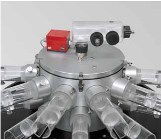
Aerosol-air mixing device with CO sensor
