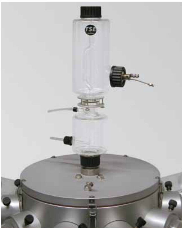
Aerosol nozzle – mounted on preseparator
