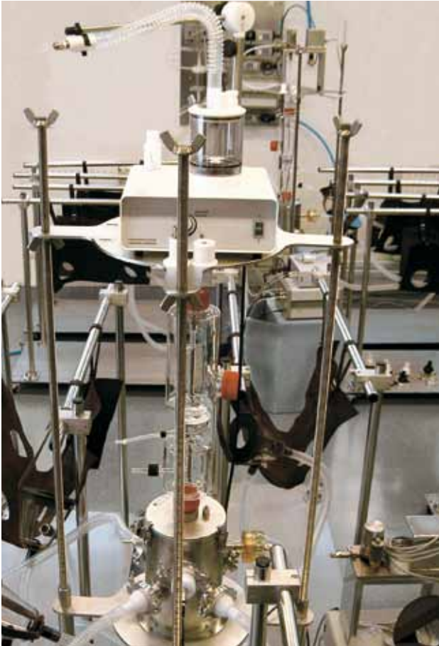
Dog Exposure Unit with ultrasonic nebulizer
