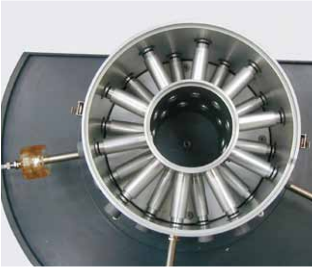
A view into the open Head Nose Only Unit from above
