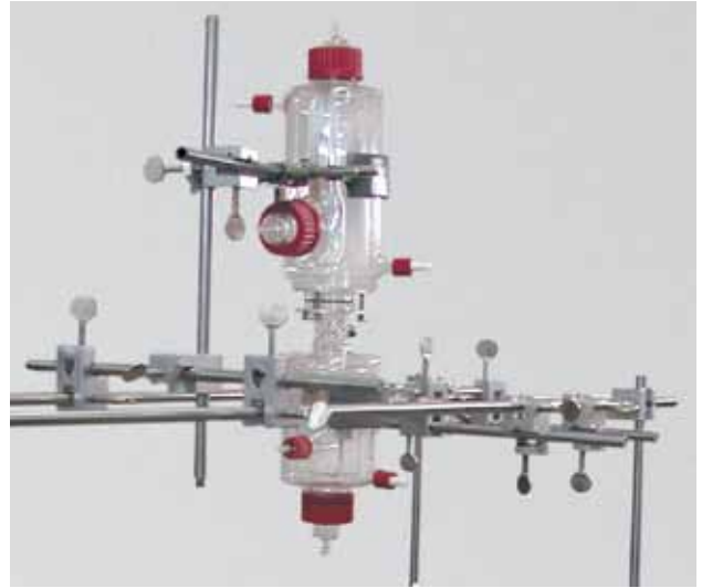
Water-jacketed mixing units for aerosol conditioning
