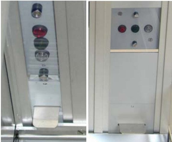
Triple stimulus lamp sets mounted over response levers Left: Mouse - vertically, Right: Rat - horizontally
