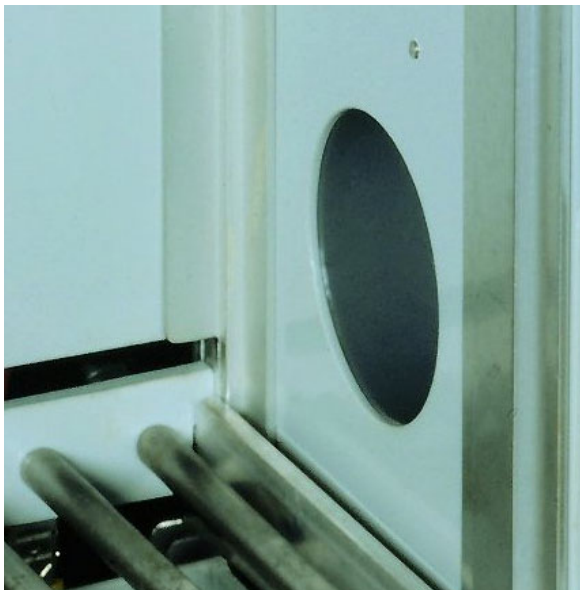
Rat nose-poke modules Circular - diameter 26mm
