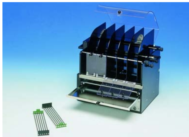
RotaRod Advanced (mice model) with floor grids, droppings collector and cover set
