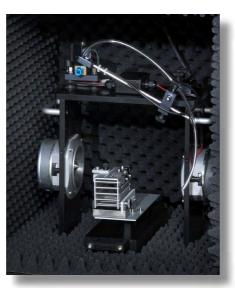
Restrainer, sensor platform & stimulus base unit in sound-attenuating housing
