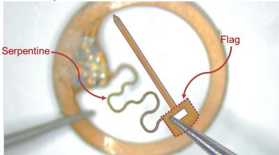
4. Using a pair of tweezers again, guide the flag onto the tooth of the clip and secure it by closing the clip down on the flag.
