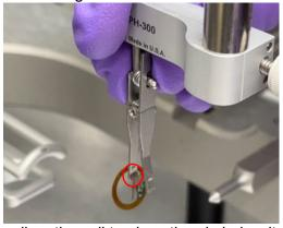
5. Use the tweezers to pull up the coil to place the pin below it.
