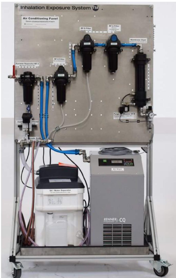
Air Conditioning Panel – compressed air filtration
