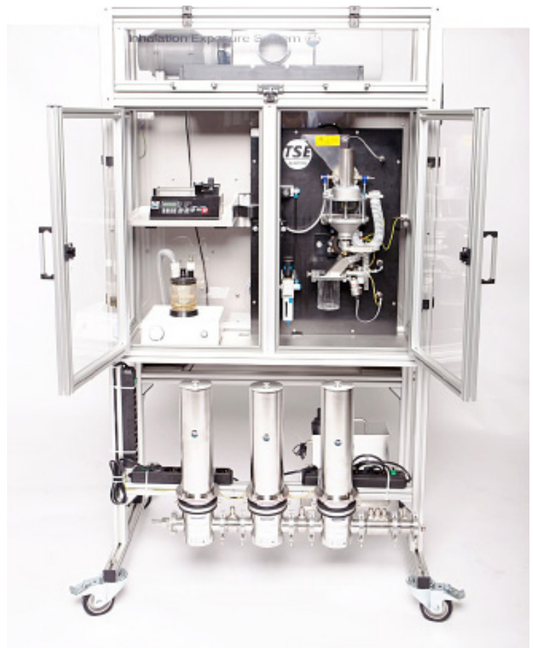
Hood, Mounting Panel (front) – Generators with additional filter system
